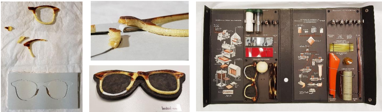
Fig. 6: Mounting the broken pieces of the Cellulose nitrate (CN) spectacle frame on acid free cardboard, dyed with plant's ash and gum Arabic, with acid free soft tissue as removable layer in contact with CN; right: fitting in the folder as a way for exhibiting
